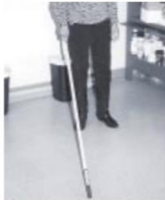
Extended handle on tool allows upright, comfortable posture
